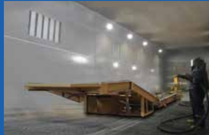
► Surface cleaned by Grit shot blasting
